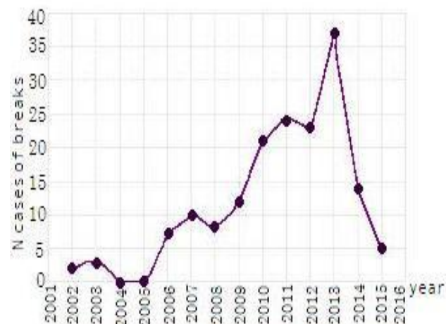
Fig.1. Statistics of breakages of side frames of bogies 18-100 per 2002 - 2015
