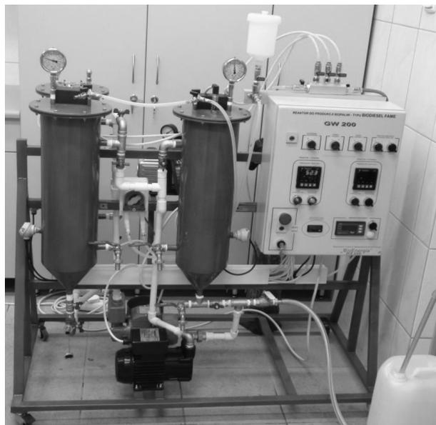
**Fig. 2.** Reactor GW 200 for production of Biodiesel FAME (CME)
