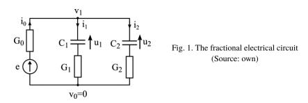
Using Kirchhoff's laws we obtain the equations describing the dynamics of tensions  $u_1(t)$ ,  $u_2(t)$  on the corresponding capacitors in response to the control voltage e(t). The corresponding circuit analysis has been concluded in [18].
