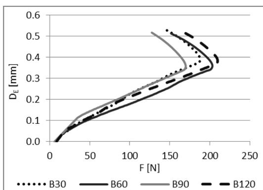
Fig. 4. Mechanical deformation curves (B-tests performed on room temperature samples)
