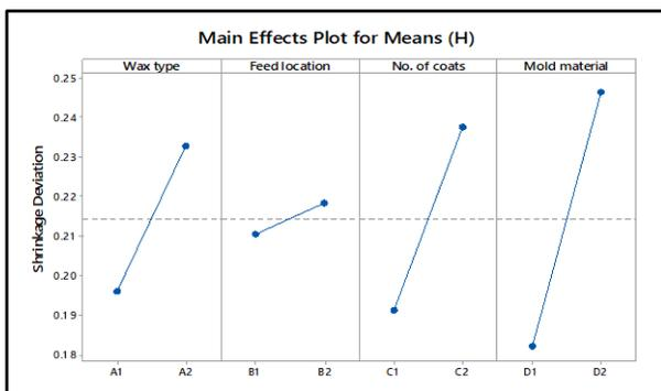
Fig. 6. Main effect of factors on shrinkage deviation of height
