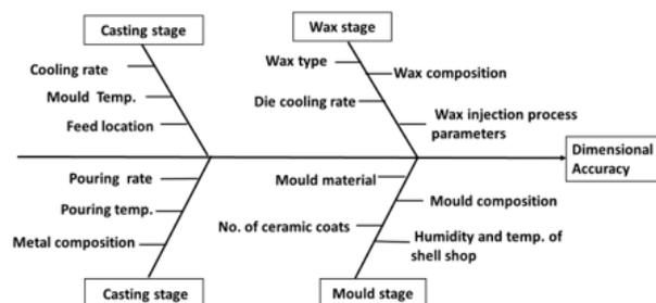
Fig. 2. Factors affecting dimensional accuracy of IC process
