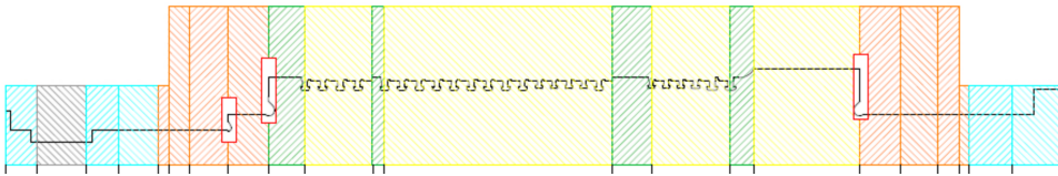
Fig. 5. Heat transfer regions in a steam turbine rotor
