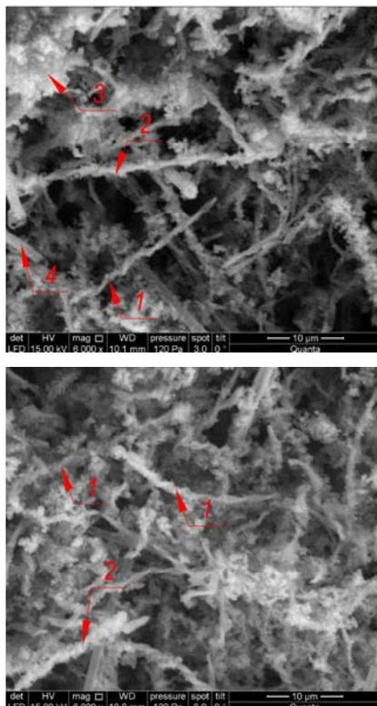
Fig. 2. Microphotographs of matrix structures of biominerals obtained with the help of scanning electronic microscope FEI Quanta; 1 = spiral-like covers of *Gallionella ferruginea*; 2 = crystalline precipitate of iron oxyhydrate on bacterial covers of *Gallionella ferruginea*; 3 = agglomerates of matrix structure; 4 = tubular structures of *Leptothrix*; 6000x; source: own study
