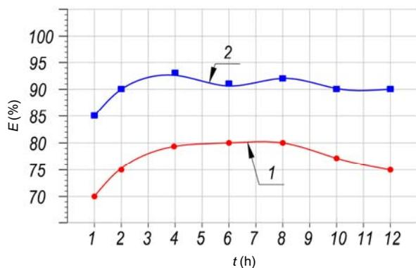
Fig. 5. Change in the efficiency ( $E$ ) of water purification throughout the filter cycle: 1 = without using additional carbon source; 2 = using the solution of soda ash;  $t$  = time; source: own study
