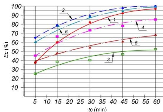
Fig. 3. The kinetics ( $E_c$ ) of the concentration ratio of  $Fe^{2+}$  ions in suspended sediment from matrix biomineral; water quality parameters of graphs 1–6 are presented in the Table 1; source: own study
