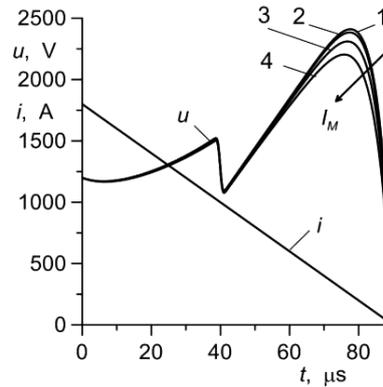
Fig. 4. Current  $i$  and voltage  $u$  curves in a circuit with the arc model (39) during circuit interruption ( $P_M = 2.2$  MW,  $\tau = 9$   $\mu$ s,  $\cot \psi = 386.1$  V/ $\mu$ s,  $U_{cr} = 1250$  V,  $i_{cr} = 1000$  A,  $\beta = 4.683 \cdot 10^{-3}$  A<sup>-2</sup>,  $G_0 = 1.5$  S) with various residual currents in the model (1 –  $I_M = 0$  A, 2 –  $I_M = 50$  A, 3 –  $I_M = 100$  A, 4 –  $I_M = 150$  A)
