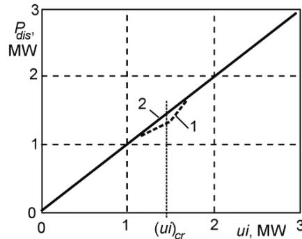
Fig. 2. Dependence of dissipated power  $P_{dis}$  on the supplied electric power  $ui$  (1 – experiment; 2 – approximation) (source: own work, based on [5])
