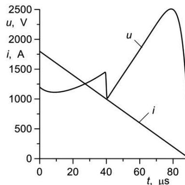
Fig. 5. Current and voltage curves in a circuit with the arc model (23) during circuit interruption ( $P_M = 2$  MW,  $\tau = 8$   $\mu$ s,  $\cot \psi = 800$  V/ $\mu$ s,  $U_{cr} = 1250$  V,  $i_{cr} = 1000$  A,  $\Delta U = 500$  V,  $G_0 = 1.5$  S,  $I_M = 10$  A)
