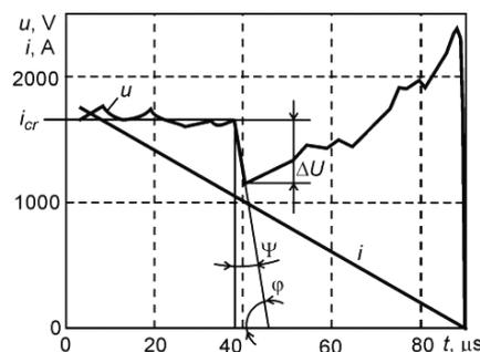
Fig. 1. Voltage  $u$  and current  $i$  curves during the circuit breaker operation
