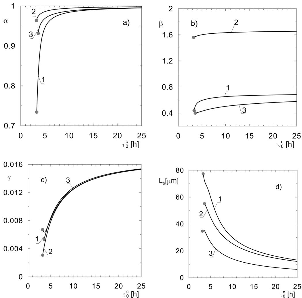
Fig. 2. Steady state branches of three-phase fluidized bed bioreactor for two values of  $\vartheta$  and two values of  $\zeta$  (glucose utilization; at grey points the condition  $u_{0c} = u_t$  is fulfilled). Lines 1 –  $\vartheta = 1.5$  and  $\zeta = 0.01$ ; lines 2 –  $\vartheta = 3.5$  and  $\zeta = 0.01$ ; lines 3 –  $\vartheta = 1.5$  and  $\zeta = 0.05$  ( $c_{Af} = 0.5 \text{ kg/m}^3$ ;  $\xi = 0.2$ ;  $\rho_0 = 1400 \text{ kg/m}^3$ ;  $u_{0g} = 0.005 \text{ m/s}$ )
