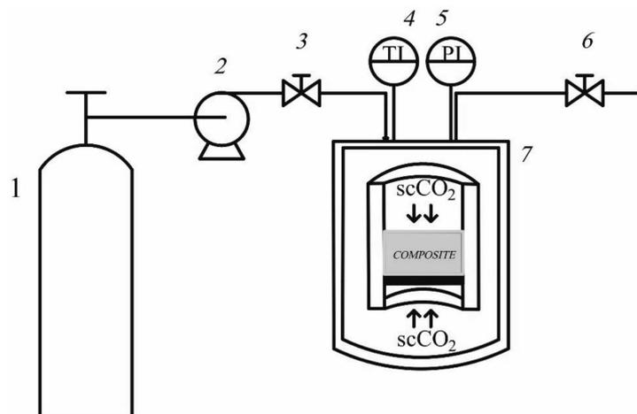
Fig. 1. Schematic diagram of the experimental system: (1) Carbon dioxide tank, (2) scCO<sub>2</sub> pump, (3) valve, (4) temperature indicator, (5) pressure indicator, (6) back pressure regulator, (7) high pressure vessel
