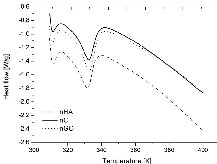
Fig. 3. DSC thermogram of composite porous structures obtained under the foaming conditions  $P_{\text{sat}} = 18 \text{ MPa}$ ,  $T_{\text{sat}} = 343 \text{ K}$ ,  $t_{\text{sat}} = 1 \text{ h}$
