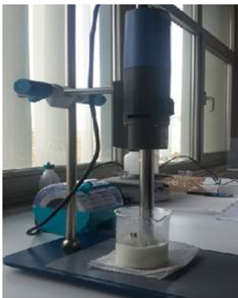
Fig. 1. High shear disperser and emulsified kerosene
