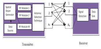
Fig.2. MIMO Wireless Communication System with Antenna Selection Technique
