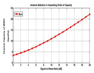
Fig.7 Channel Capacity of MIMO when fourth antenna (M=4) is selected.
