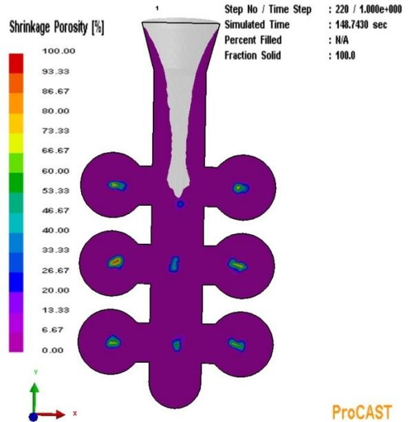
Fig.3. The result of the distribution of shrinkage defects across the section
