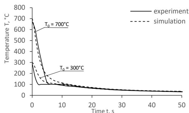
Fig. 8. Comparison of the results of numerical calculations and experimental tests for cooling in water (22°C) from the initial temperature of 700°C and 300°C
