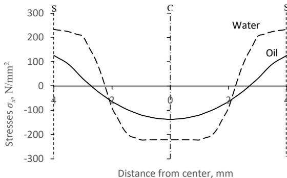
Fig. 11. Distribution of stresses  $\sigma_x$  on the cross-section of the rib after time  $\Delta t$  at cooling from  $700^\circ\text{C}$  to  $22^\circ\text{C}$
