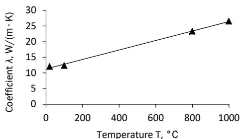
Fig. 5. Thermal conductivity coefficient vs temperature for cast 1.4849
