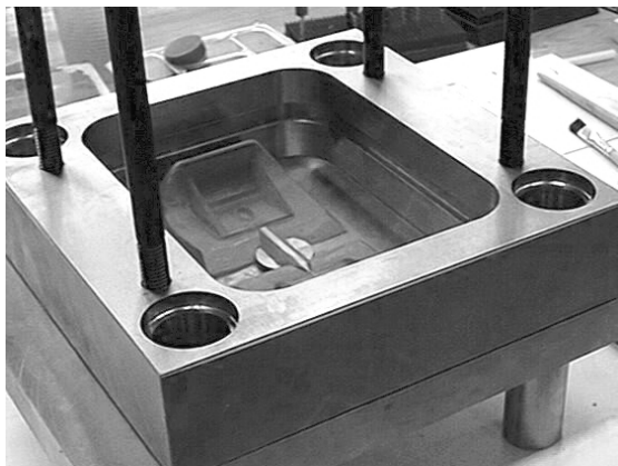
Fig. 20. View of a model with shaped parting plane, fixed in the mould frame
