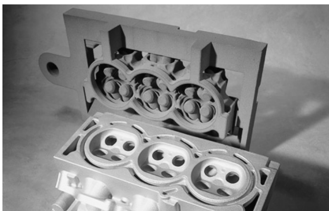
Fig. 8. V6 Cylinder head for 24-valve car engine Integrated sand cores, produced in one piece, for fully functional cast prototypes in AlSi9Cu3 Material: quartz 4.2 Courtesy of: VAW Südalumin and Becker CCC, Germany
