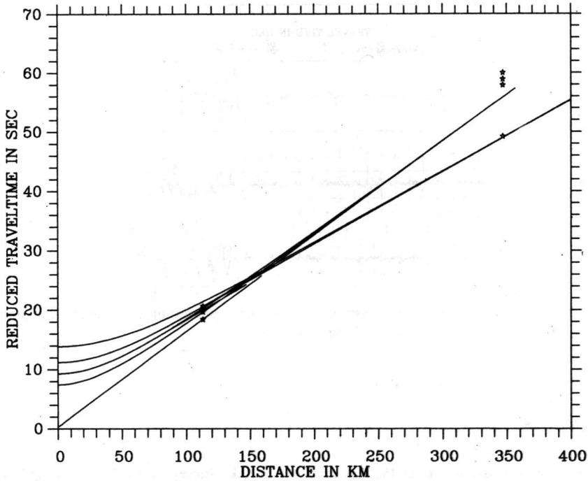
Fig. 7. The travel-time calculated for distance 0—400 km (crust model fig. 3, asterisks — phases read from the seismograms)
