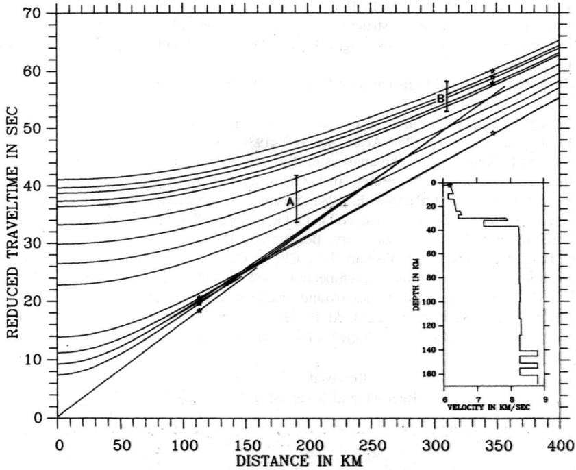
Fig. 8. The travel-time calculated for kinematic model with horizontal discontinuities at depth of 150 km (asterisks — phases read from the seismograms)
