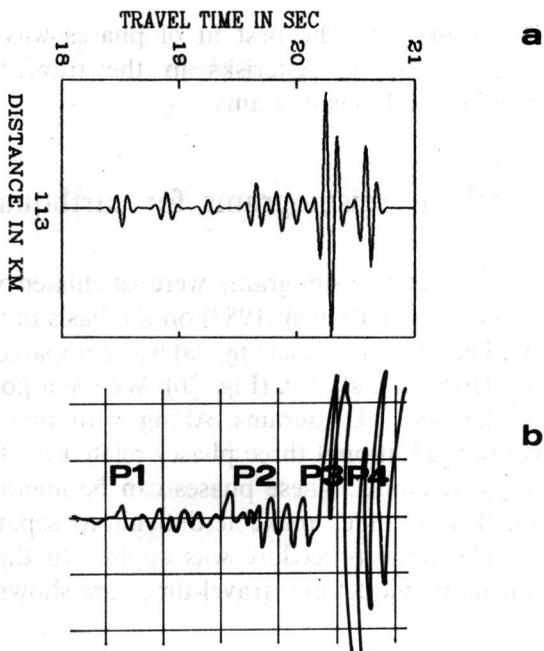
Fig. 2. Comparison of the seismogram recorded at the *Hornsund* Station (b) and the synthetic seismogram (a)
