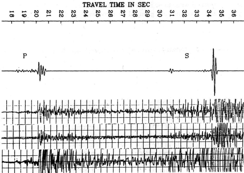
Fig. 5. Comparison of the synthetic seismogram calculated for P-S waves and the seismograms recorded at the *Hornsund* Station
