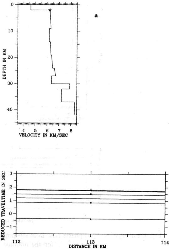
Fig. 3. Fitting of phases P1-P4 read from the seismogram (asterisks) to the travel-time (b) calculated for the adopted model (a)
