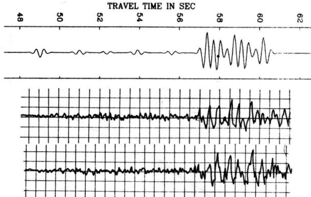
Fig. 9. Comparison of the synthetic seismogram and the seismograms recorded at the *Hornsund* Station (P waves)
