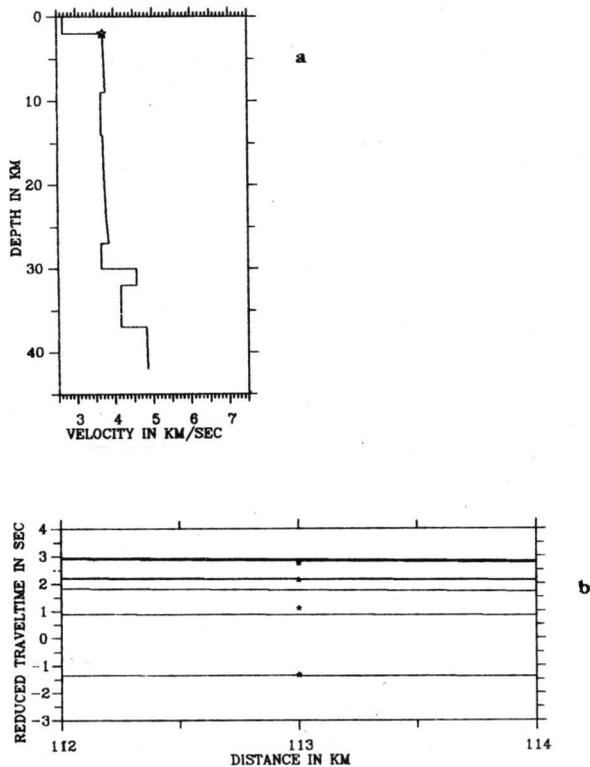
Fig. 4. Fitting of S waves phases read from seismogram (asterisks) to the travel-time (b) calculated for the adopted model (a)
