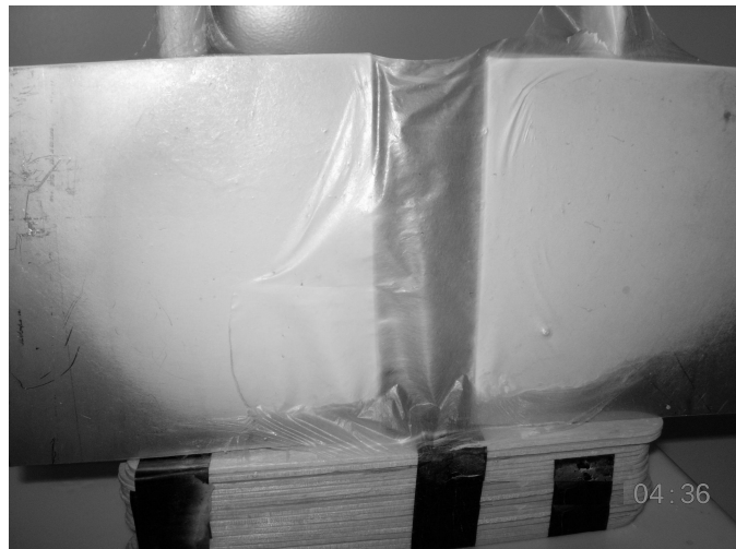
Fig. 3. Collection of the wafer-like non-woven mat of the as-spun Al_2O_3 -PVP composite
