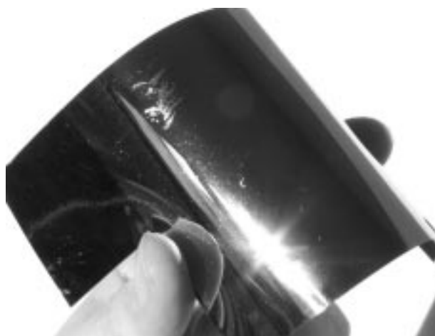
Fig. 8. Test structure of elastic CdTe layer based on UPILEX® foil and contacted by 2µm Cu layer
