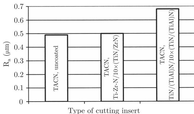
Fig. 6. Average values of roughness parameter  $R_a$  of the rollers machined with the TACN grade ceramic cutting inserts, coated and uncoated
