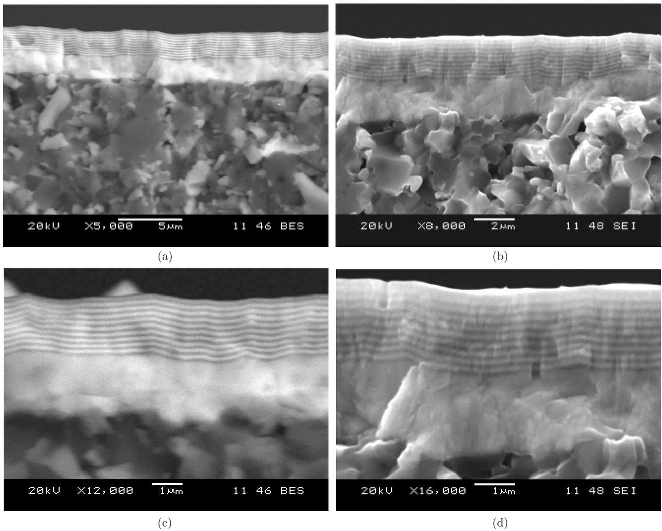
Fig. 1. SEM micrographs showing the fractured multilayer Ti-Zr-N/  $10\times$  (TiN/ZrN) coating deposited on TACN grade ceramic cutting insert at different magnifications and types of electron image:  $5000\times$ , BES (a),  $8000\times$ , SEI (b),  $12000\times$ , BES (c) oraz  $16000\times$ , SEI (d)
