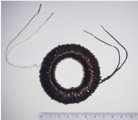
Fig. 1. Measuring sample for magnetic properties
