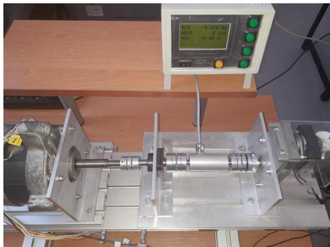
Fig. 9. Measuring stand for determination of SRM torque
