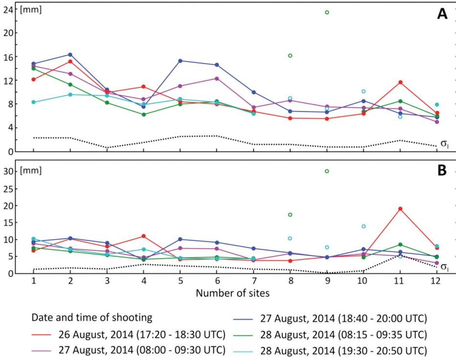
Fig. 7. Index of average grain size (A) and sorting (B); dotted line – standard deviation of the index at study sites; points without filling – incorrect result data Sedimetrics® Digital Gravelometer.
