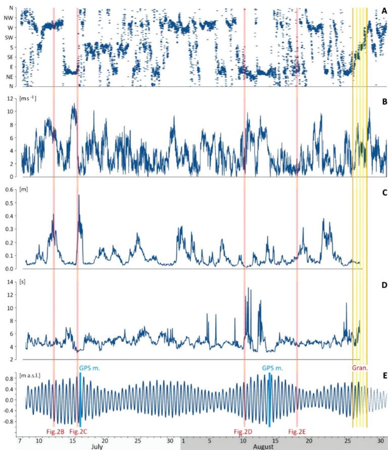
Fig. 5. Data from the summer season of 2014 in the Calypsobyen: (A) wind directions, (B) wind speeds, (C) significant wave height, (D) mean wave period, and (E) height of tidal waves; solid line – data from MIDAS WTR, dotted line – simulation data. GPS m. – the date of GPS measurements of shoreline (see Fig. 6), Gran. – the date of taken of images (see Figs 7 and 8).
