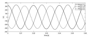
Fig. 3. The waveform of the instantaneous phase voltage at the terminals of the generator
