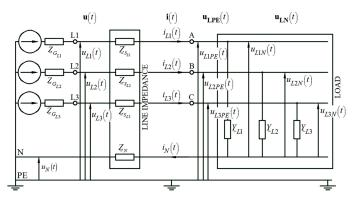
Fig. 1. Power-supply system with indicated asymmetrical sinusoidal voltage vectors
