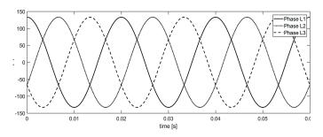
Fig. 12. The waveform of the instantaneous value of the current after compensation
