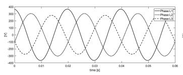
Fig. 5. The waveform of the instantaneous phase voltage at the load
