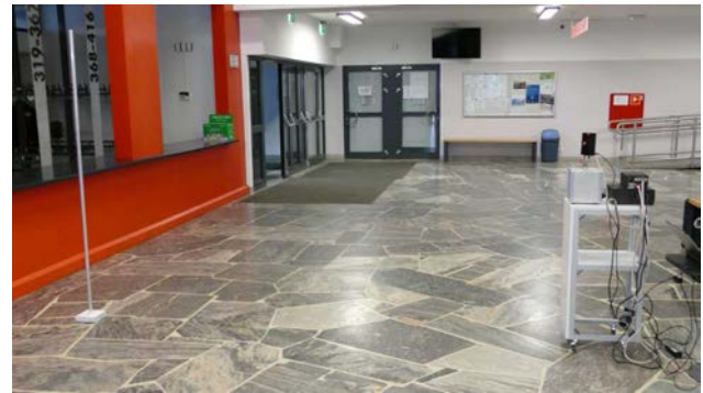
Fig. 28. Location of the rotary base with the sonar module in relation to the post at a distance of 3.4 m.
