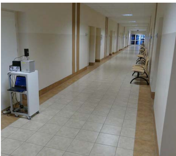
Fig. 22. Location of the rotary base with the sonar module in relation to the wall.
