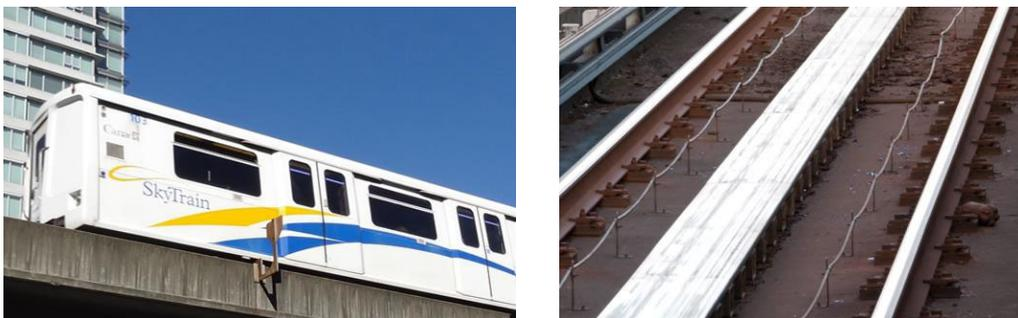
Fig. 1. SkyTrain car (left) and its reaction rail (right)
