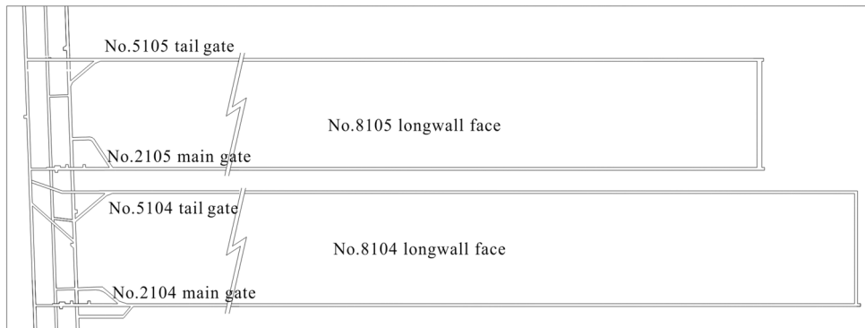
Fig. 2. Layout of No.8104 and No.8105 longwall faces
