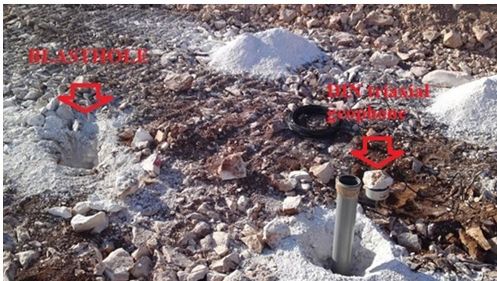
Fig. 5. The vibration monitoring instrument installation during measurement at closest point (1.5 m)
