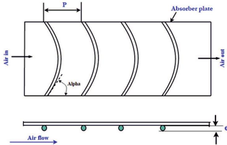
Figure 2: Geometry of wire rib roughness on the absorber plate.
