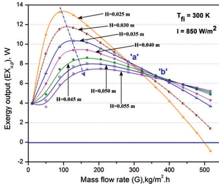
Figure 8: Variation of exergy output rate ( $EX_{u,p}$ ) as a function of mass flow rate for different values of duct depth ( $H$ ).
