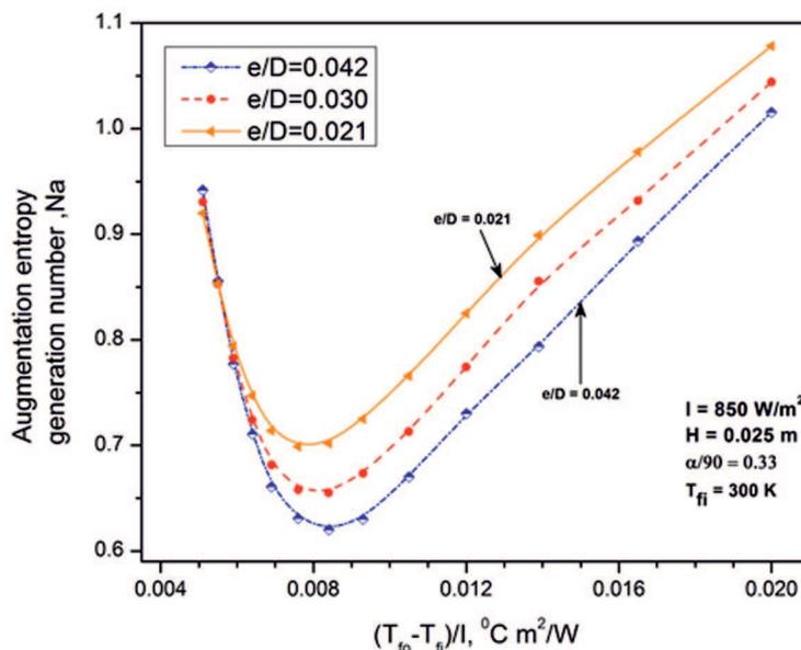
Figure 9: Variation of augmentation entropy generation number ( $Na$ ) with temperature rise parameter  $(T_{fo}-T_{fi})/I$  for different values of  $e/D$ .
