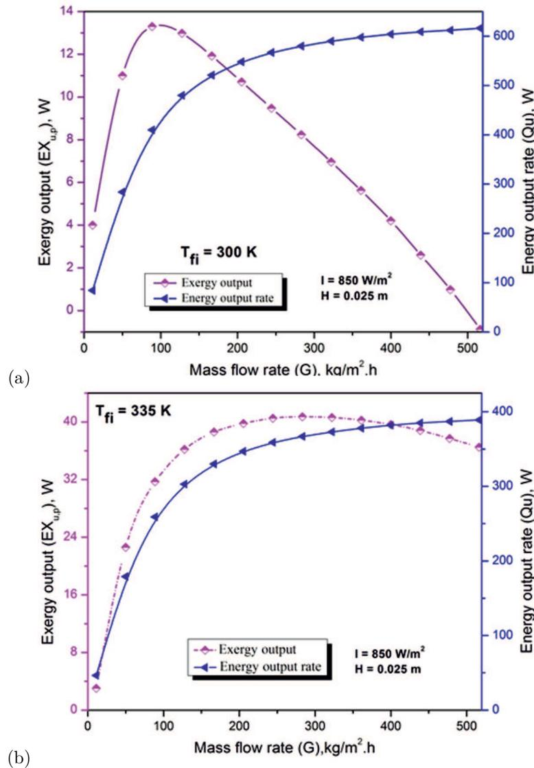
Figure 5: Variation of exergy output rate ( $EX_{u,p}$ ) and energy output rate ( $Q_u$ ) with mass flow rate ( $G$ ) at (a)  $T_{fi} = 300 \text{ K}$ , (b)  $T_{fi} = 335 \text{ K}$ .
