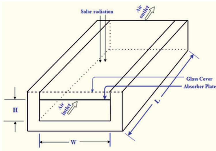
Figure 1: Solar air heater duct with simple absorber plate.
