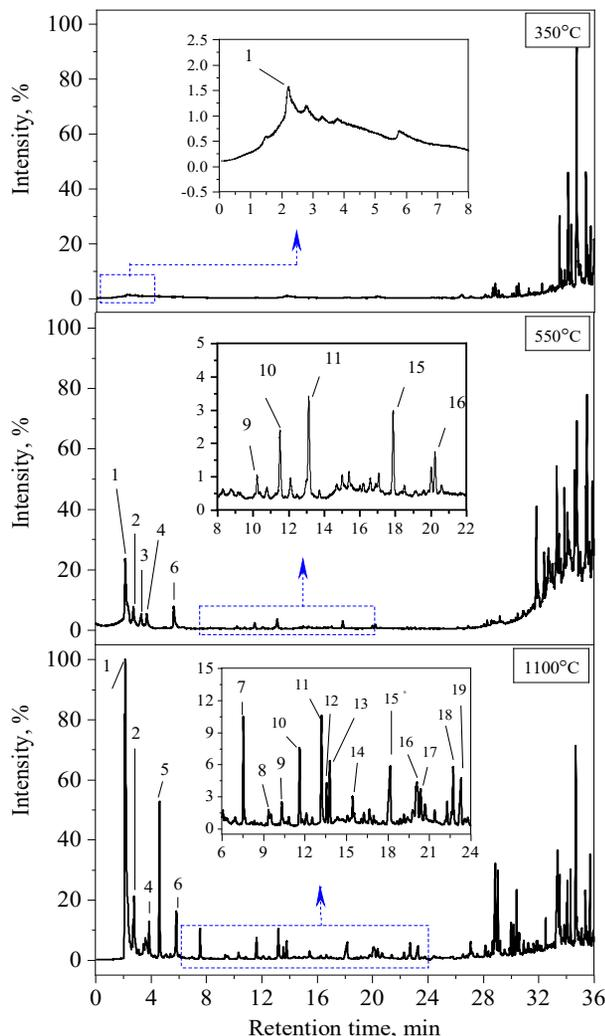
Fig. 3. Py-GC/MS chromatograms of Albertine F/1 under the different pyrolysis temperature
