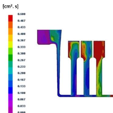
Fig. 9. Oxide occurrence – naturally pressurized gating system
