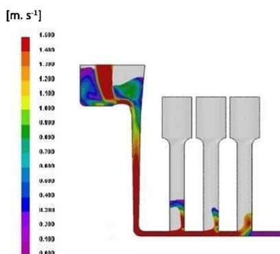
Fig. 13. Metal spatter – naturally pressurized gating system
