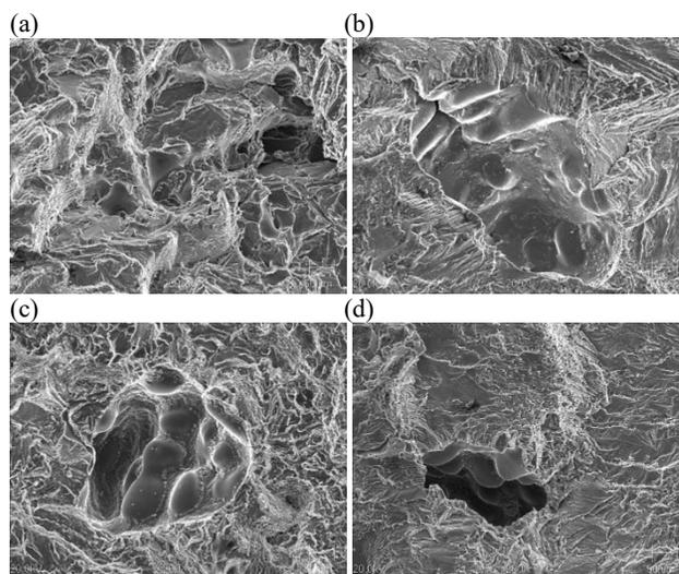
Fig. 8. Fatigue fracture surfaces of heat-treated (hyperquenching: 6 h at 540°C / water 20°C; aging: 175°C / 8 h / air) specimens of AlSi7Mg alloy subject to: (a) Process I; (b) Process II; (c) Process III; (d) Process IV
