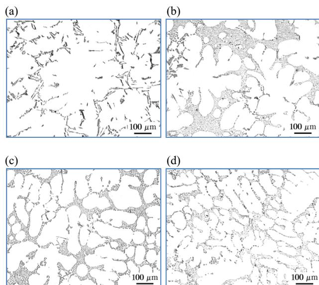
Fig. 1. AlSi7Mg alloy microstructure after: (a) refining with  $C_2Cl_6$  (Process I); (b) refining with  $C_2Cl_6$  followed by modification with Ti, B and Na (Process II); (c) refining by purging with argon and parallel modification with Ti salts, B salts, and Sr (Process III); and (d) refining by purging with argon and parallel modification with Ti, B, and Na (Process IV)
