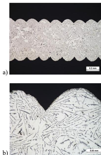
Fig. 3. Microstructure of single wall of aluminium alloy honeycomb element (a), surface of casting with topography after 3D printing pattern (b)
