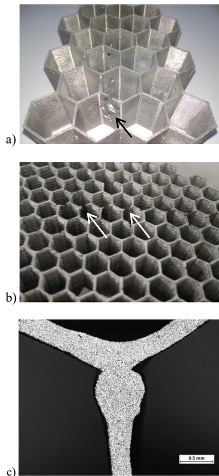
Fig. 1. Perforated walls of incorrect cast honeycomb (a, b), the connection of the three walls (c)
