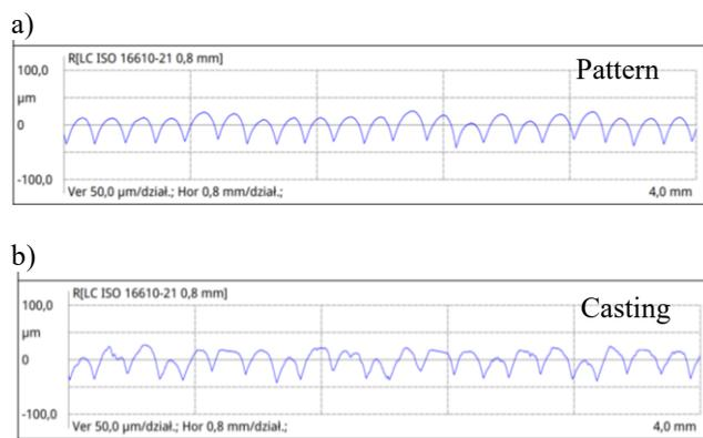
Fig. 2. Surface linear profiles for pattern made by Fused Deposition Modeling (a) and aluminium casting reproduced from polymer pattern (b)
