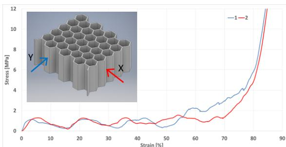
Fig. 5. Stress-strain curves of the cast honeycomb specimens with two orientation of honeycomb channels to load direction
