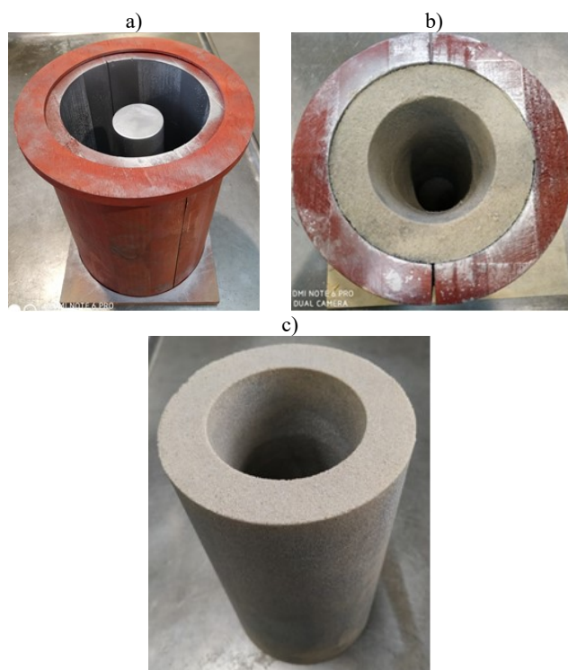
Fig. 6. Individual stages of mould making for ablation casting: a - wooden flask, b - mould resting in the flask, c - mould ready for pouring
