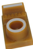
Fig. 6. Hardness test places (marked in white)
