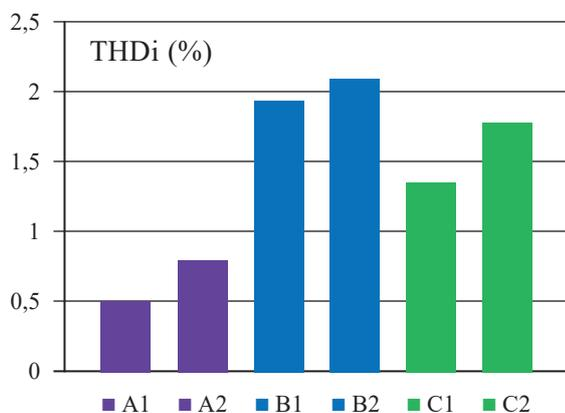
Fig. 10. Total harmonic distortion – current  $THD_i$
