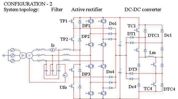
Fig. 4. System topology with three-level DC-DC converter and three-level 3-phase active rectifier
