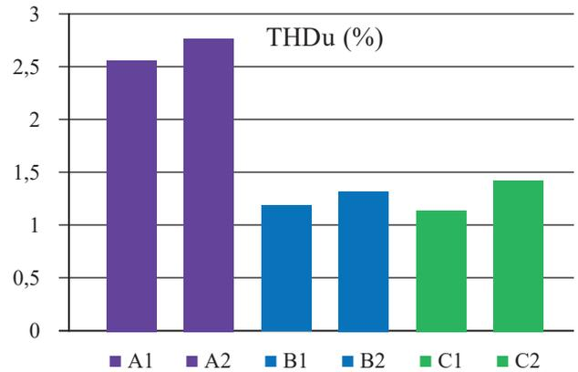
Fig. 11. Total harmonic distortion – voltage  $THD_u$
