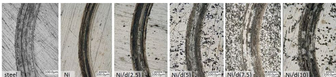
Fig. 10. Images of abrasion traces on the coating surfaces after ball-on-disc studies
