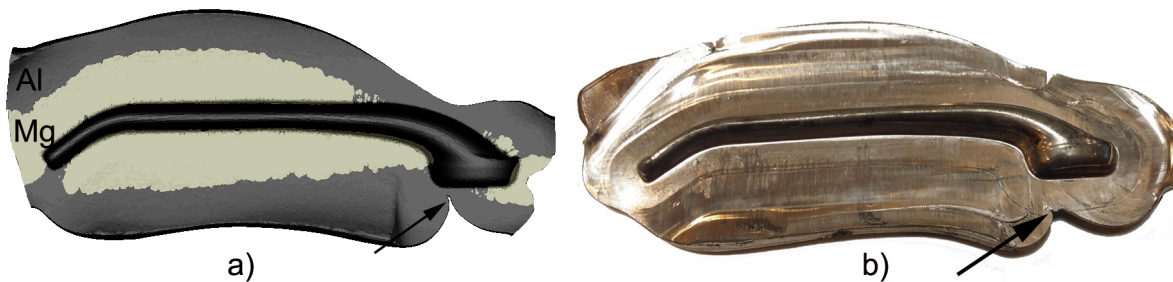
Fig. 6. Shape of forgings obtained in the numerical modelling (Variant I) – a) and experiment – b)
