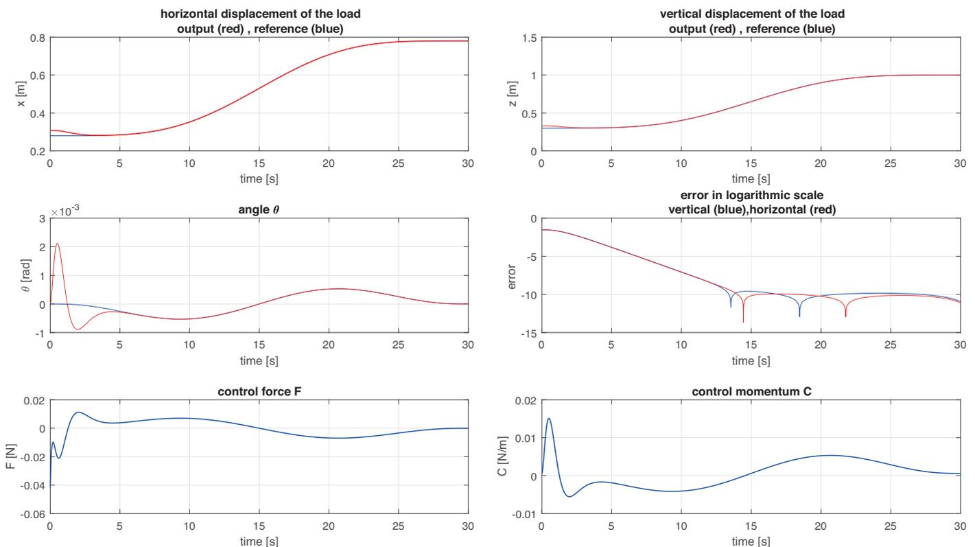
Fig. 2. Simulation results for 2-crane system (S1)
