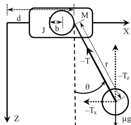
Fig. 1. The overhead two dimensional crane control system
