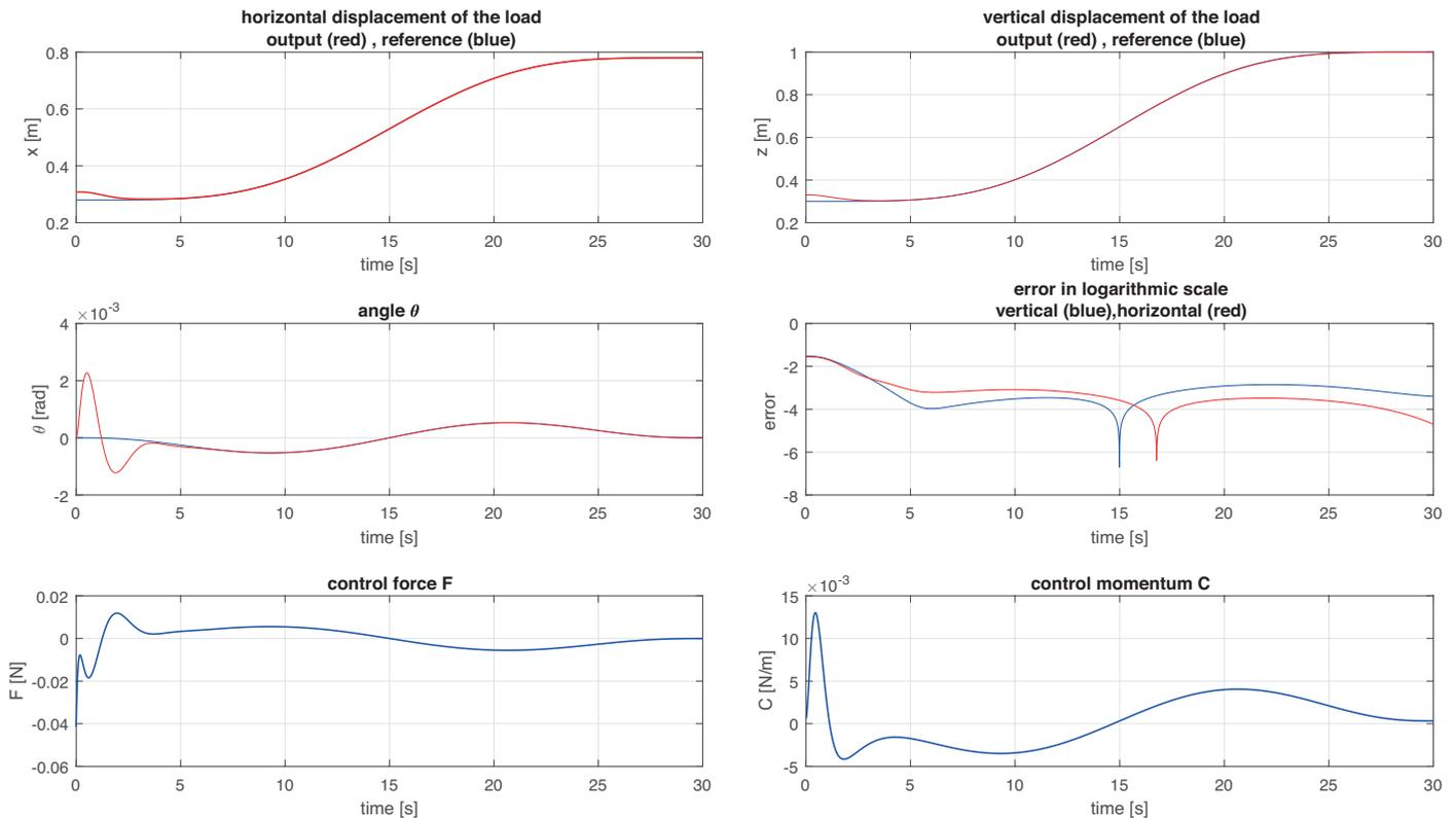
Fig. 3. Simulation results for 2-crane system with parametrical uncertainties (S2)
