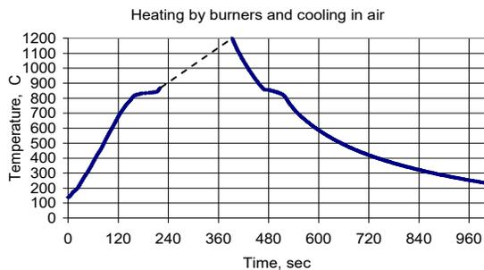
Fig. 7. Heating and cooling curve for study no.1 (specimen 1)
