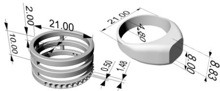
Fig. 2. Elements designed in Rhinoceros 6: ring and signet ring (geometries used in final simulations)
