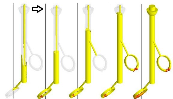
Fig. 5. Visualization of 4 stages of simulation after changing parameters according to Table 2 (almost complete filling of mould cavities was achieved).
