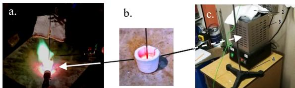
Fig. 6. Elements of workplaces for thermal analysis: a - propane-butane burners, b - 15 cm<sup>3</sup> ceramic crucible and K-type thermocouple, c - laboratory furnace with capacity of 1200W, T<sub>max</sub> = 1150°C
