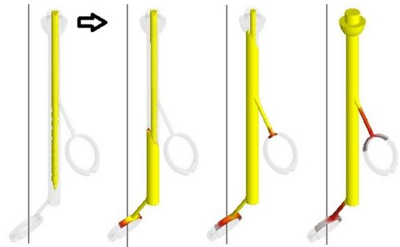
Fig. 4. Visualization of 4 stages of the process simulation, indicating the unexpectedly rapid course of solidification at the end of filling and the formation of misruns in both elements (the metal has solidified before filling the mould cavity )
