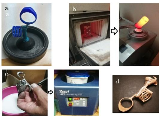
Fig. 11. View of the stages of raw casting production: a - resin model, b - burning and mould pouring, c - cleaning and polishing of the cast, d - raw casting after cleaning
