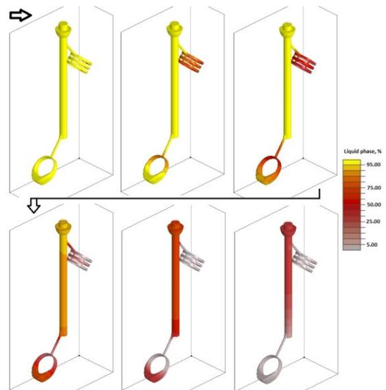
Fig. 9. Selected stages of simulation of solidification of ring and signet out of Au-Ag-Cu alloy (+Zn), discretization grid Δx = 0.5 mm
