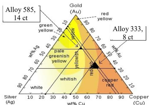
Fig. 1. Ternary plot of approximate colors of Ag–Au–Cu alloys [7,19]
