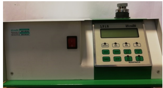
Fig. 7. LPiR device for measuring the permeability of Multiserw company
