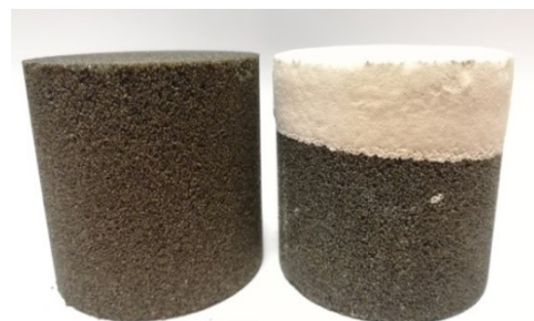
Fig. 4. Cylindrical profiles with the dimensions \Phi 50 \times 50 mm before and after applying a protective coating
