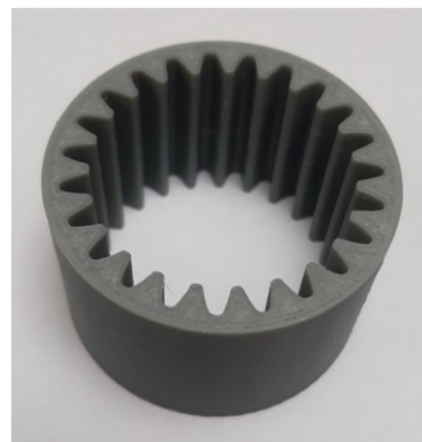
Fig. 4. The female mould for the ceramic preform
