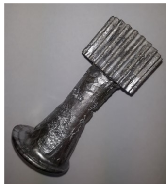
Fig. 8. Composite casting with the gating system
