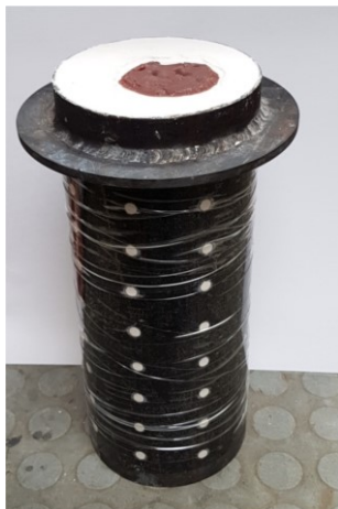
Fig. 6. The mould prepared for firing
