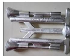
Fig.1. Test bar and its casting
