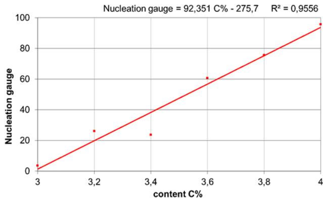
Fig. 5. Influence of carbon level on nucleation gauge
