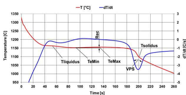
Fig. 1. Specific temperatures and VPS coefficient in the derivative-thermal analysis (DTA)
