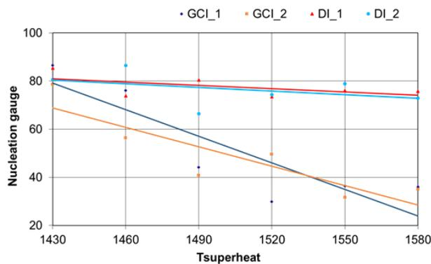
Fig. 14. Influence of overheating temperature on nucleation gauge
