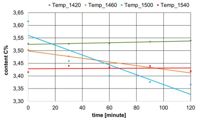
Fig. 9. Influence of holding time and temperature on cast iron carbon level
