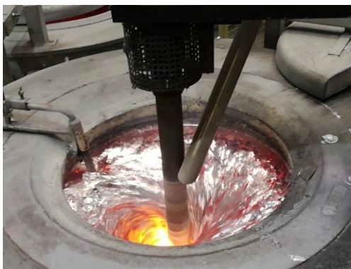
Fig. 1. Flux addition during rotary degassing
