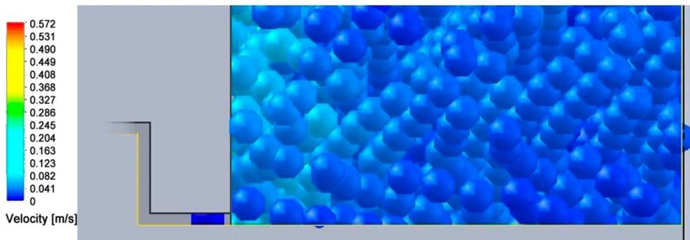
Fig. 7. Simulation of particles falling into the labyrinth seal
