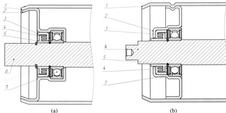
Fig. 2. General construction of bearing roller: a) locked by rolling; b) locked by bending: 1 – roller housing, 2 – bearing housing, 3 – labyrinth seal, 4 – contact seal, 5 – ring, 6 – shaft, 7 – bearing
