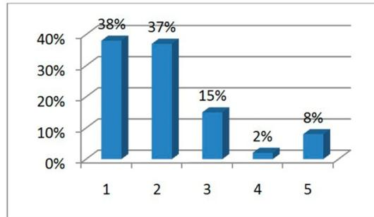
Fig. 1. Statistical distribution of bearing failures: 1 – clogging, 2 – lack of or insufficient lubrication, 3 – relaxation of interference fit, 4 – wear of the body during overloads, 5 – other
