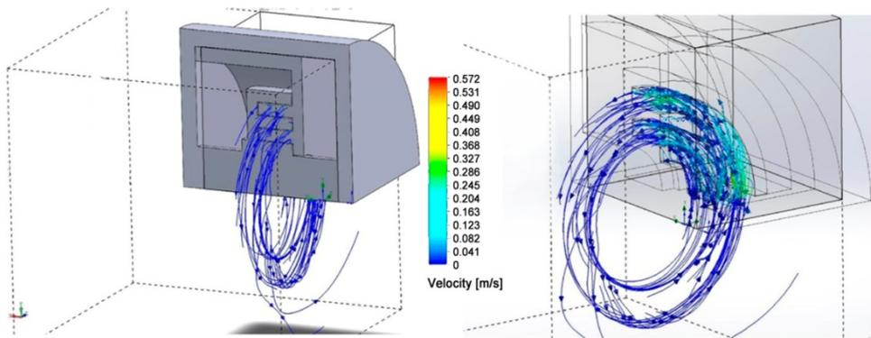
Fig. 6. Lines of airflow in the gap of the labyrinth seal
