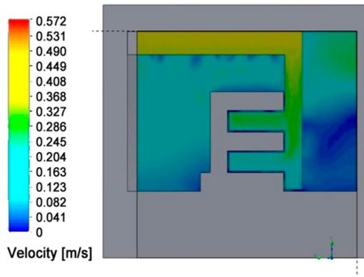
Fig. 4. Airflow velocity around the labyrinth seal
