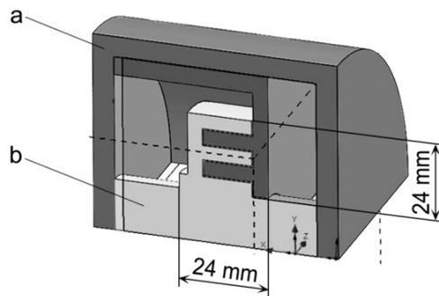
Fig. 3. Seal model: a – rotating part, b – fixed part
