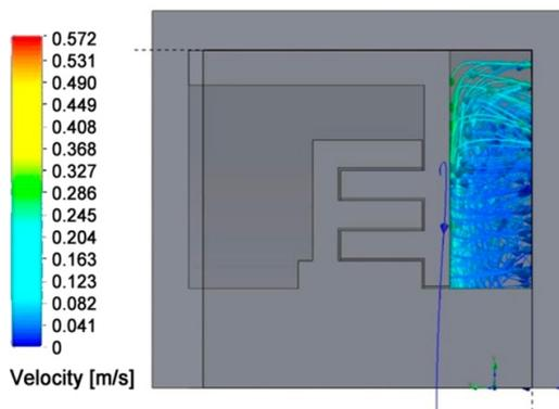
Fig. 5. Lines of airflow from the outside of the labyrinth seal
