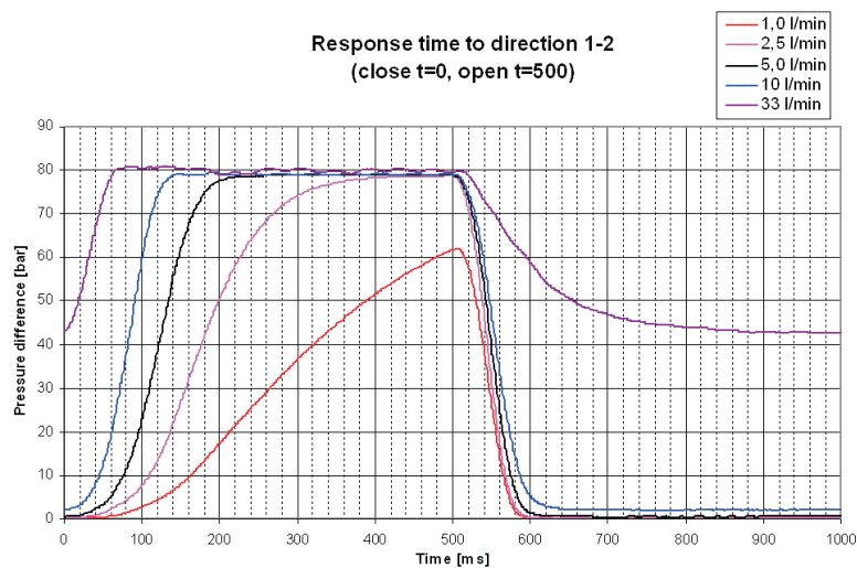
Fig. 5. Valve response time in flow direction from port 1 to 2 (rebound)
