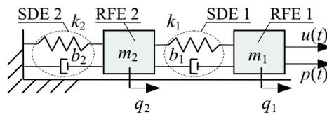
Fig. 2. Model of the structure under consideration
