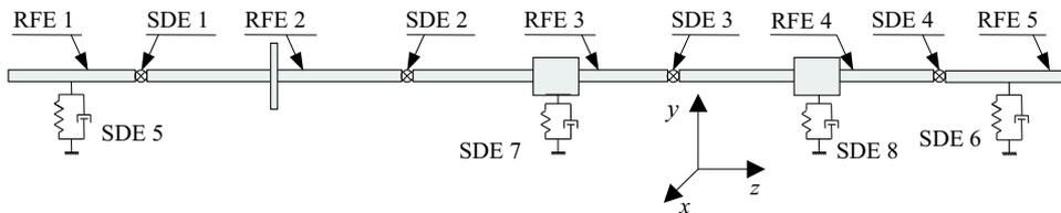
Fig. 5. The discrete model of the laboratory rotor
