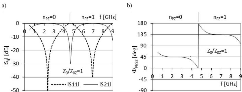
Fig. 6. The amplitude characteristics (a), and the differential phase shift  $\Phi_{\text{PhSZ}}$  (b), of a microwave phase shifter with a parallel short-circuited stub for  $Z_0/Z_{0Z} = 1$  (results of simulations,  $L_{\text{Ref}} = 74.5$  mm).
