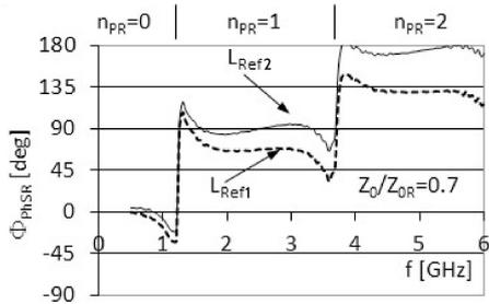
Fig. 14. The measured differential phase shift  $\Phi_{PhSR}$  of a microwave phase shifter with a parallel open-circuited stub for  $Z_0/Z_{0R} = 0.7$  and for two various reference line lengths ( $L_{Ref1} = 80$  mm,  $L_{Ref2} = 88.7$  mm).
