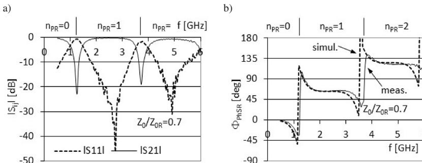
Fig. 11. The measured amplitude characteristics (a), and the differential phase shift  $\Phi_{PHSR}$  (b), of a microwave phase shifter with a parallel open-circuited stub for  $Z_0/Z_{0R} = 0.7$  ( $w_{SR} = 1.37$  mm,  $L_{SR} = 35$  mm,  $L_{Ref} = 80$  mm).
