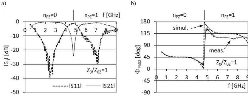
Fig. 12. The measured amplitude characteristics (a), and the differential phase shift  $\Phi_{PhSZ}$  (b), of a microwave phase shifter with a parallel short-circuited stub for  $Z_0/Z_{0Z} = 1$  ( $w_{SZ} = 2.73$  mm,  $L_{SZ} = 17$  mm,  $L_{Ref} = 74.5$  mm).
