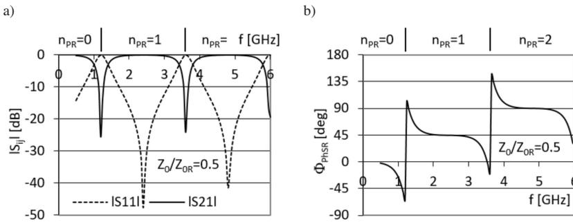
Fig. 4. The amplitude characteristics (a), and the differential phase shift  $\Phi_{\text{PhSR}}$  (b), of a microwave phase shifter with a parallel open-circuited stub for  $Z_0/Z_{0R} = 0.5$  (results of simulations,  $L_{\text{Ref}} = 74.5$  mm).
