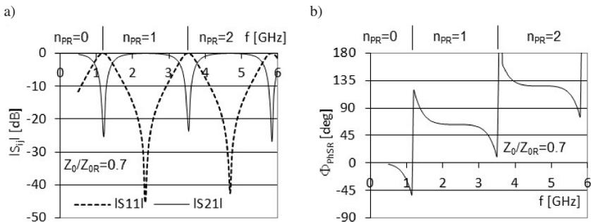
Fig. 5. The amplitude characteristics (a), and the differential phase shift  $\Phi_{\text{PhSR}}$  (b), of a microwave phase shifter with a parallel open-circuited stub for  $Z_0/Z_{0R} = 0.7$  (results of simulations,  $L_{\text{Ref}} = 80$  mm).
