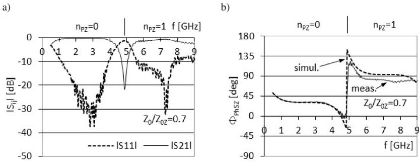
Fig. 13. The measured amplitude characteristics (a), and the differential phase shift  $\Phi_{PhSZ}$  (b), of a microwave phase shifter with a parallel short-circuited stub for  $Z_0/Z_{0Z} = 0.7$  ( $w_{SZ} = 1.36$  mm,  $L_{SZ} = 17$  mm,  $L_{Ref} = 70$  mm).
