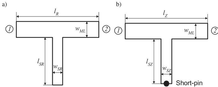
Fig. 8. Schematic views of the phase shifters with single parallel stubs made in microstrip technology, a) with an open-circuit stub; b) with a short-circuit stub.
