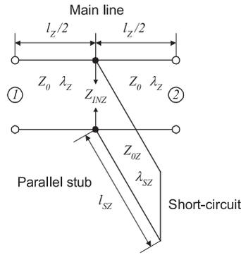
Fig. 3. A microwave phase shifter with a single parallel short-circuited stub.
