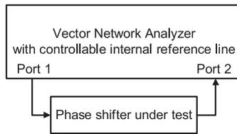
Fig. 9. A schematic block diagram of the measurement setup of phase shifters.
