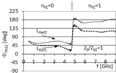
Fig. 15. The measured differential phase shift  $\Phi_{\text{PhSZ}}$  of a microwave phase shifter with a parallel short-circuited stub for  $Z_0/Z_{0Z} = 1$  and for two various reference line lengths ( $L_{\text{Ref1}} = 74.5$  mm,  $L_{\text{Ref2}} = 80.5$  mm).
