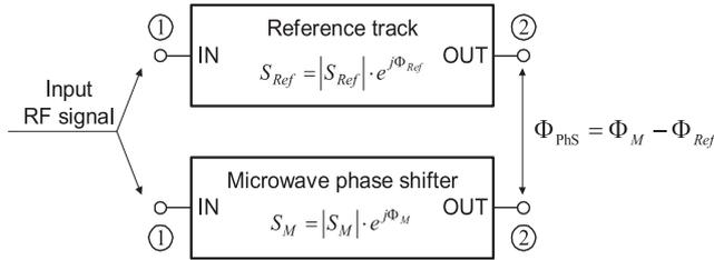
Fig. 1. A symbolic composition of a microwave phase shifter and a reference track to demonstrate *differential phase shift*  $\Phi_{\text{PhS}}$ .
