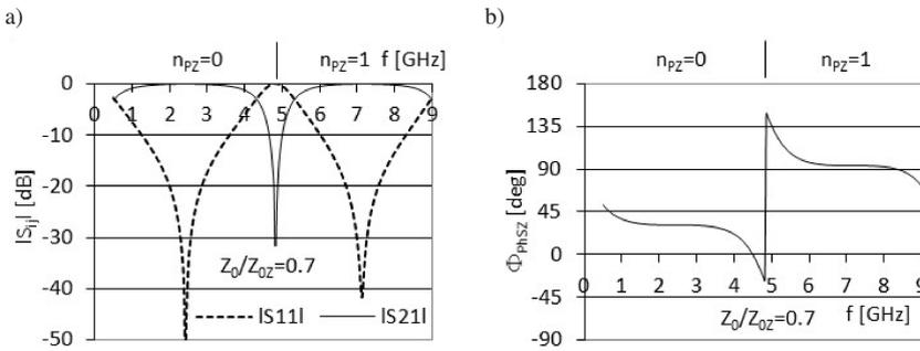
Fig. 7. The amplitude characteristics (a), and the differential phase shift  $\Phi_{PhSZ}$  (b), of a microwave phase shifter with a parallel short-circuited stub for  $Z_0/Z_{0z} = 0.7$  (results of simulations,  $L_{Ref} = 70$  mm).
