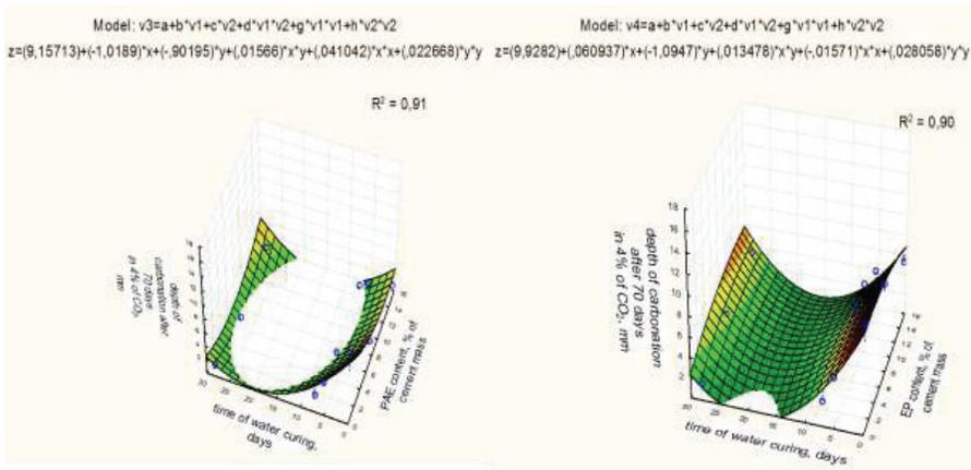
Figure 13. Depth of carbonation after 70 days of exposure in 4% CO<sub>2</sub> atmosphere as a function of time of water curing and polymer content
