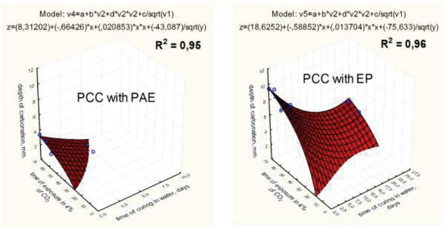
Figure 14. Models of carbonation progress in time for PCC concretes with PAE and EP polymers
