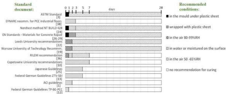
Figure 1. Time of PCC curing in humid conditions by various recommendations assuming 28 days as the time of total maturing.
