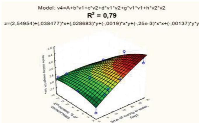
Figure 6. Tensile splitting strength for 28-days old PCC with PE as a function of PE content and water curing time
