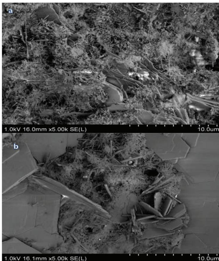
Figure 12 SEM analysis of microstructure of 28-days old polymer-cement concrete with 15% of EP after different regimes of curing: a) 14 days in wet conditions (water) and 14 days in dry conditions; b) 28 days in dry conditions
