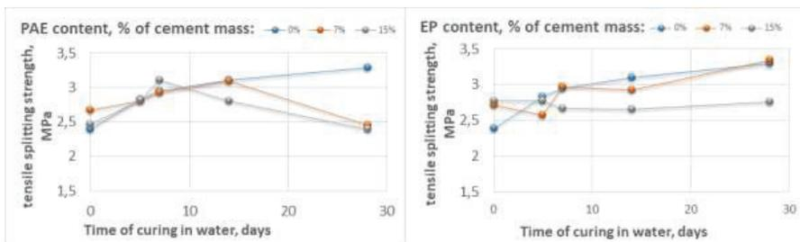
Figure 4. Effect of water curing time on tensile splitting strength of PCC with PAE (a) and EP (b). Test performed for 28-days old concrete
