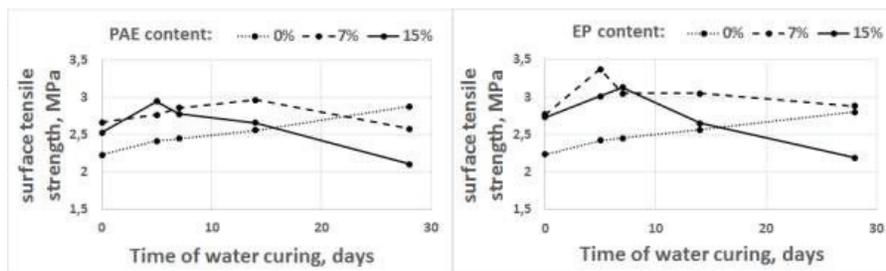
Figure 7. Effect of water curing time on surface tensile strength of a PCC with PAE (a) and EP (b). Test performed for 28-days old concrete
