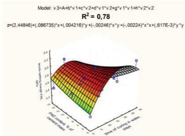
Figure 5. Tensile splitting strength for 28-days old PCC with PAE as a function of PAE content and water curing time
