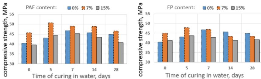
Figure 3. Influence of water curing time on the compressive strength of concrete. Test performed for 28 days concrete
