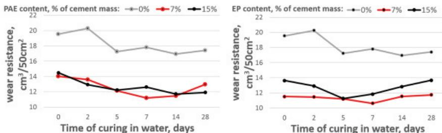
Figure 9. The influence of water curing time on wear resistance of a PCC with PAE (a) and EP (b). Test performed for 28-days old concrete
