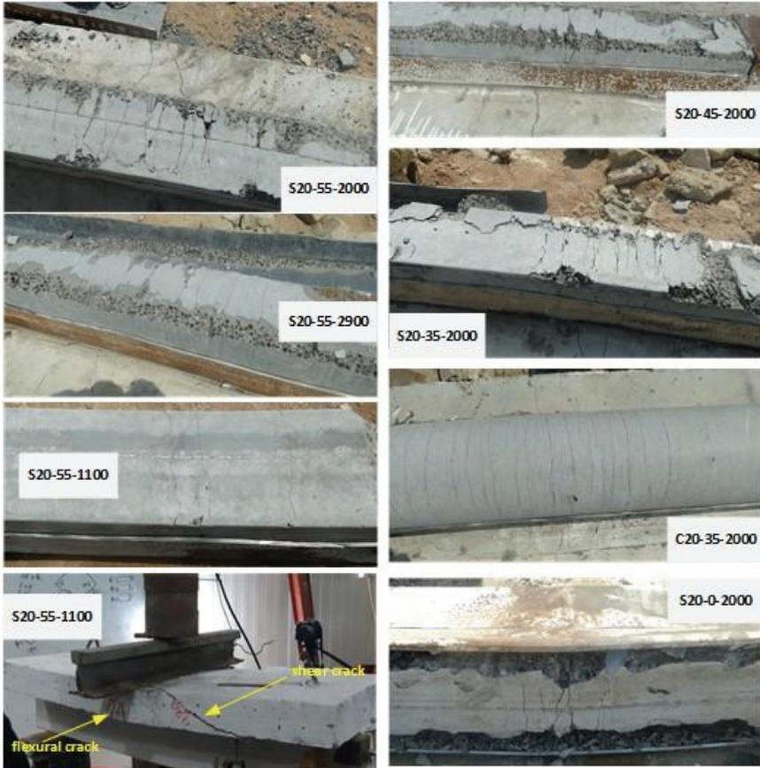
Fig. 6. Cracks in the test specimens.
