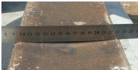
Fig. 11. Buckling of the bottom flange for specimen S0-55-2000.
