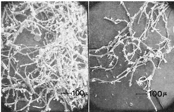
Fig. 11. Cluttered aramide fibres after mastification [31]
